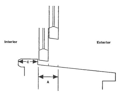
Side view of window (with no storm window) showing window trough area, A, to be tested. Trough is strip across window sill where interior window sashes can touch the sill. The interior window sill is shown as area C. Interior window sills and window troughs should be sampled separately.
