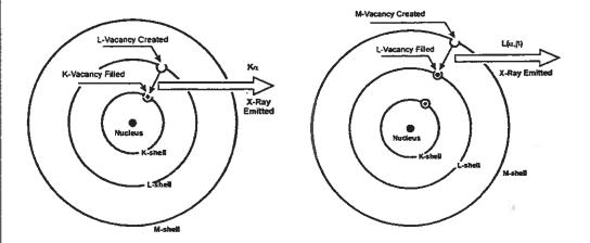
Figure 5-3. Illustration of electron shell vacancies and filling
