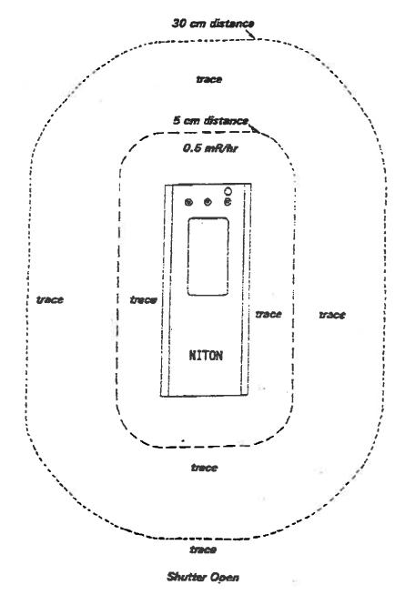
Max radioactivity on operator's hand, with shutter open: 0.05 mR/hr Trace = < 0.06 mR/hr - Not detectable above natural background levels.
